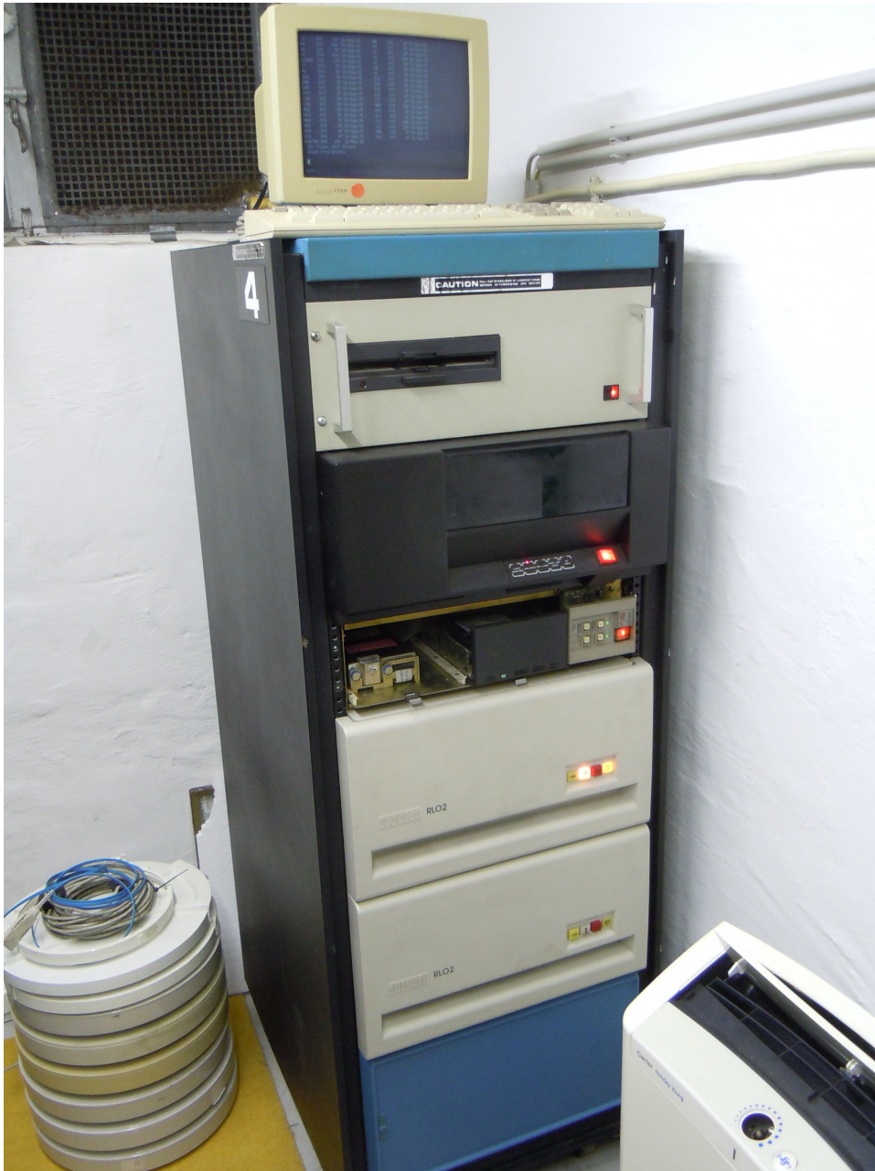
Figure 1: The destination system – a QBUS PDP11 that thinks it is a PDP11/84
